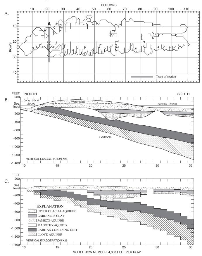
**Figure 8.** Horizontal and vertical discretization using deformed layers for the model simulating ground-water flow on Long Island, New York: (A) horizontal grid, (B) hydrogeologic cross section, and (C) vertical grid using deformed layers. (Modified from Buxton and others, 1999.)
