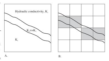
**Figure 4.** Large finite-difference cells may be inadequate to represent some important features of a ground-water system. (A) Map of the distribution of horizontal hydraulic conductivity showing a channel of high hydraulic conductivity. (B) Finite-difference cells representing the high hydraulic-conductivity channel are no longer continuous, because there is no direct connection between diagonal cells in the finitedifference method.
