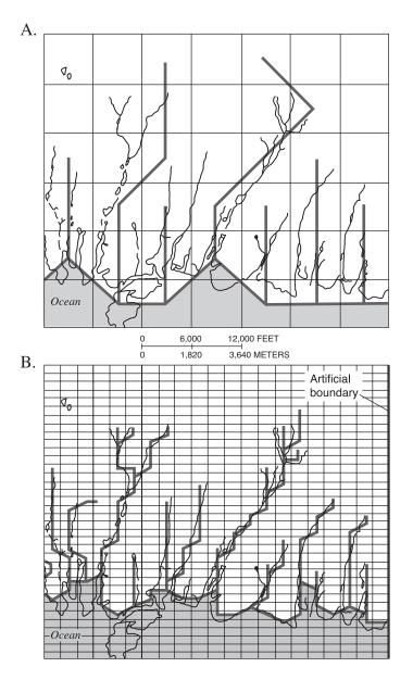
**Figure 2.** Representation of stream and shoreline boundaries on Long Island, New York, (A) as represented in a regional groundwater flow model grid, and (B) as represented in a sub-regional ground-water flow model grid. (Modified from Buxton and Reilly, 1987.)
