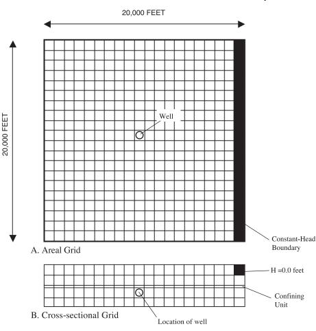
**Figure 13.** Extent and model grid of the finite-difference model used to illustrate initial conditions: (A) areal grid, and (B) cross-sectional grid.
