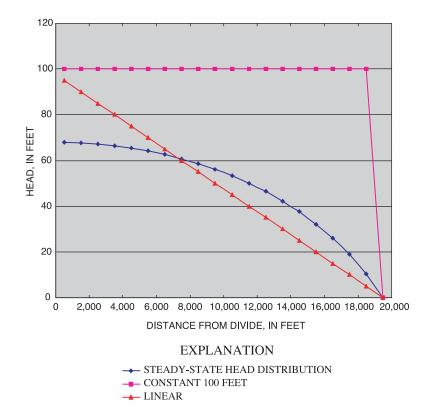
**Figure 14.** Head distribution along a model row from the divide to the constant-head node for three different initial conditions used for a transient simulation.
