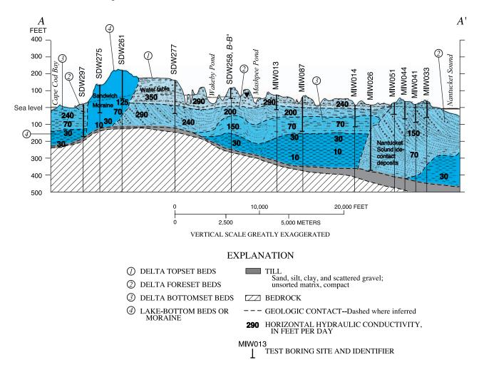
**Figure 7B.** Horizontal and vertical discretization using uniform layers for the model simulating ground-water flow on Cape Cod, Massachussetts. Hydrogeologic cross section near column 85. (Modified from Masterson and others, 1997.)
