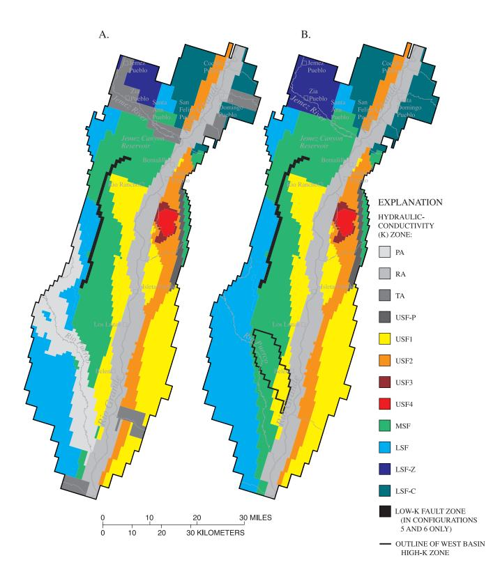
**Figure 18.** Hydraulic-conductivity zones identified for automatic parameter estimation in a ground-water flow model of the Albuquerque Basin, New Mexico: (A) zones in model layer 1, and (B) zones in model layer 2. (From Tiedeman and others, 1998.)
