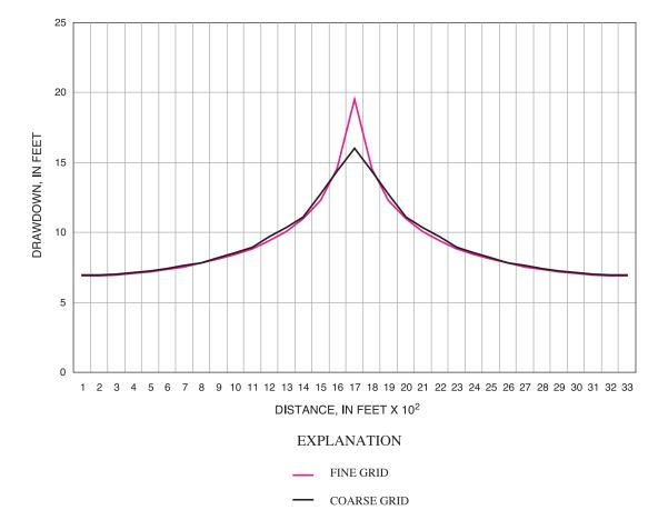
Figure 5. Cross section of drawdown showing the effect of grid spacing.
