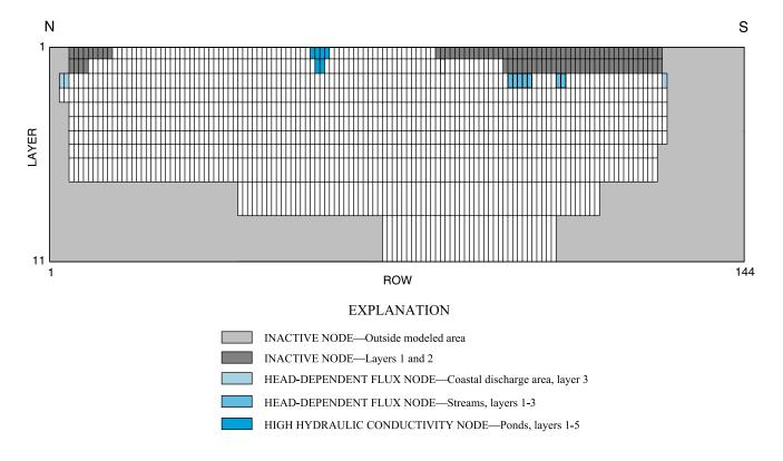
**Figure 7C.** Horizontal and vertical discretization using uniform layers for the model simulating ground-water flow on Cape Cod, Massachussetts. Vertical grid using uniform layers along column 85. (Modified from Masterson and others, 1997.)
