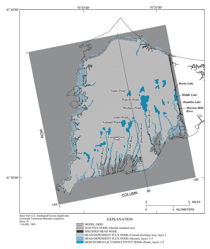
**Figure 7A.** Horizontal and vertical discretization using uniform layers for the model simulating ground-water flow on Cape Cod, Massachussetts. Horizontal grid. (Modified from Masterson and others, 1997.)
